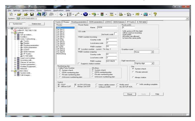
In Routing Parameters make sure that **No, and type, outgoing** is set to **PABX Number**.
