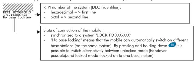
Note: The `locked' mode makes it easier to determine the area covered on a specific BS.
