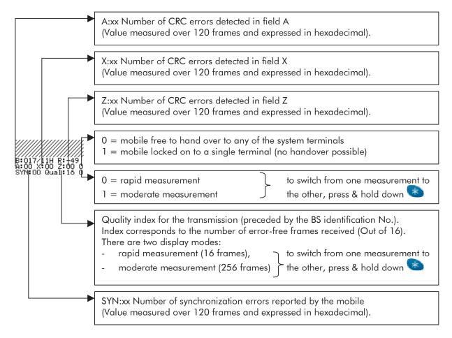
Note: the quality index gives an objective overview of the quality of the link, enabling the practical range to be determined (these depend both on the distance of the handset and the type of environment). In practice, the best procedure is to select this function (preferably in moderate measurement), make a call and note the value of the index (Q): at a given location the quality can be considered good if the value displayed remains stable at 12 or above.
