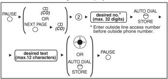
Similar to the above procedure, when storing other types of buttons (CO buttons, feature buttons, etc.), the displayed text for the Self Labelling LCD Display can be assigned.
